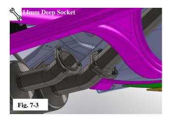
(f) Install the two new gaskets, supplied in the kit, on the TRD center muffler assembly rear (outlet) pipes for tailpipe installation.
